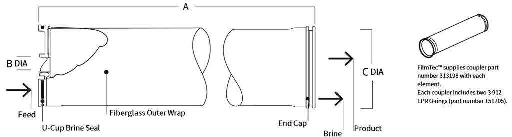
FilmTec™ supplies coupler part number 313198 with each element. Each coupler includes two 3912 EPR O-rings (part number 151705).
